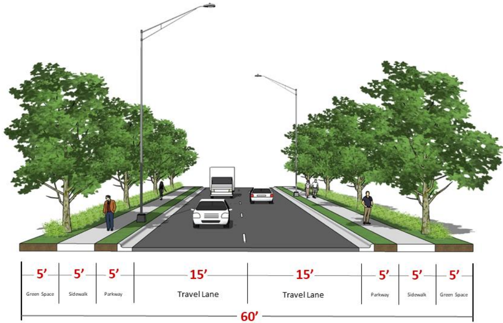
Minor Urban/Commercial Collector – 2 Lane, 60' ROW, 15' Lanes
